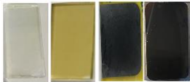
TCO Substrate CdS coated TCO Sb 2 Se 3 film side view Sb 2 Se 3 glass side view
