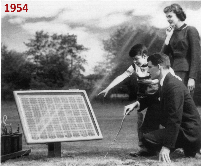
1954 Something New Under the Sun. It's the Bell Solar Battery, made of thin discs of specially treated silicon, an ingredient of common sand. It converts the sun's rays directly into usable amounts of electricity. Simple and trouble-free. (The storage batteries beside the solar battery store up its electricity for night use.)
