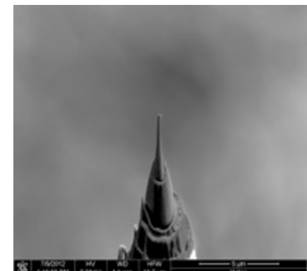
6. Final FIB shaping of specimen
