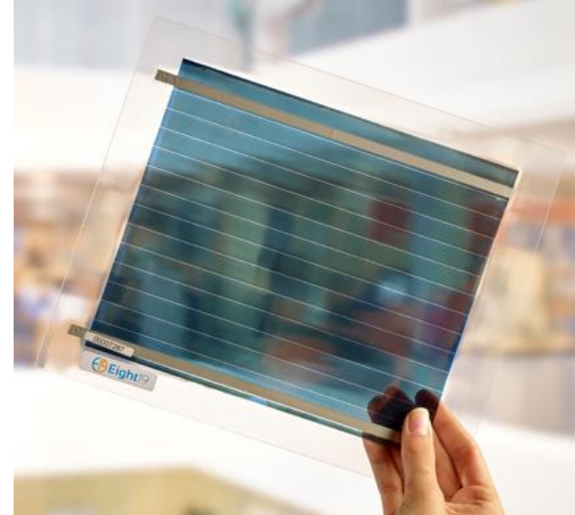
A low temperature screen-printed organic PV module. Cheap to make, transparent, bendable.
