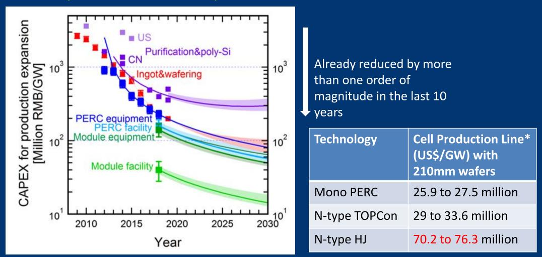
The PV Industry is capable to grow PERC capacity even with low Gross Margin
