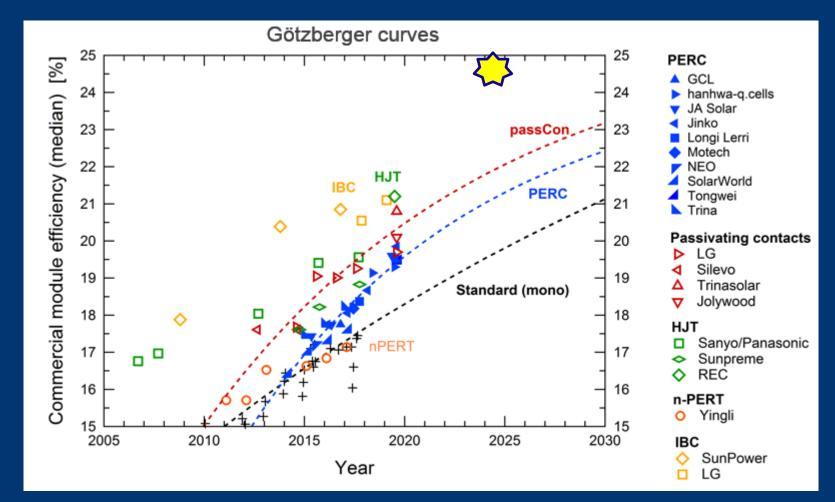
… Silicon-based Tandem cells with efficiency > 26% will soon be
