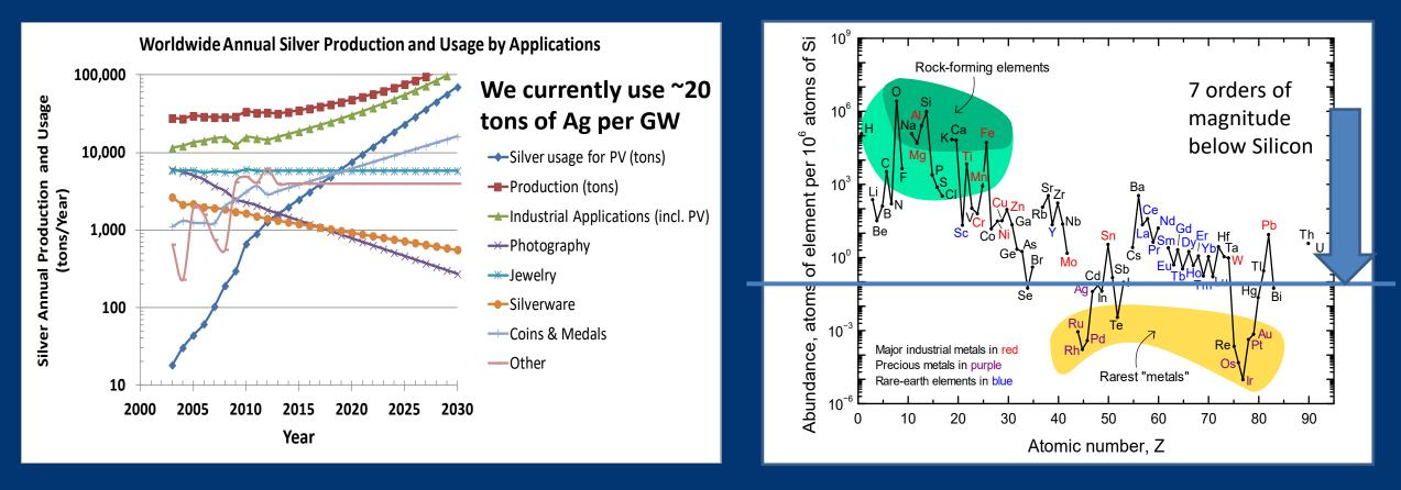
World Production of Ag ~ 30,000 Tons p.a. Recycling does not become significant until 2050. At 3TW p.a. (~2040), the usage of Ag must be < 5mg/W (currently ~ 20mg/W)
