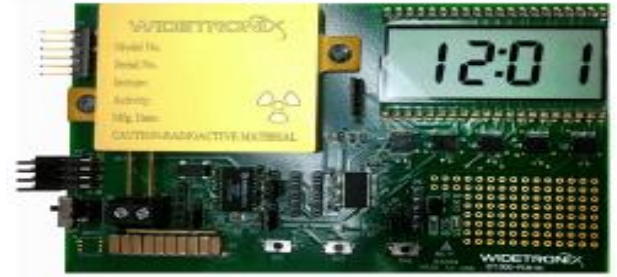
Power supply of sensor
