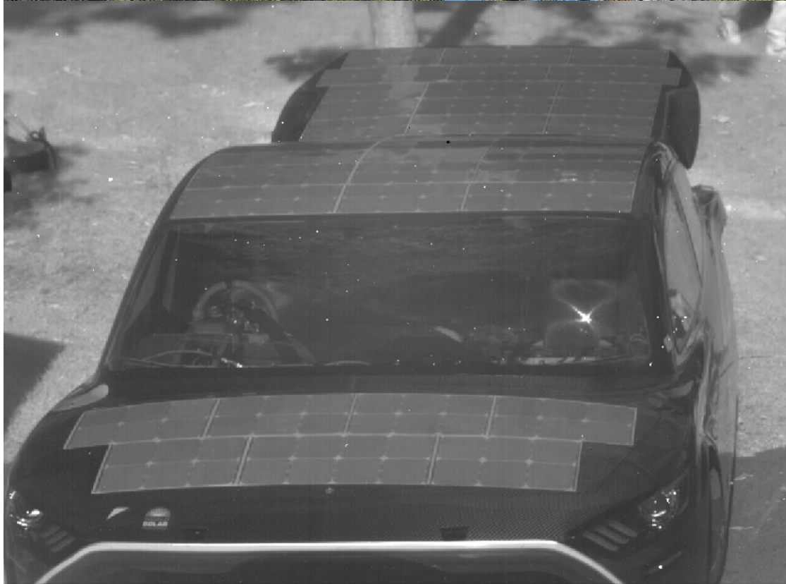
Outdoor PL imaging demonstration on the UNSW solar car
