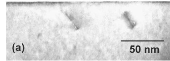
(a) Cross-sectional TEM micrographs of single crystal silicon, viewed in a \langle 110 \rangle projection.
