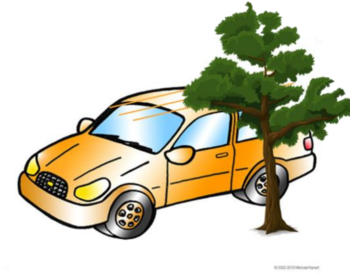
Partial shading (Parking) Inherent mismatching by a partial shading
