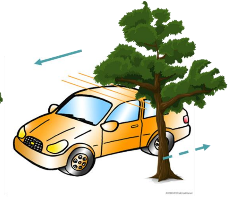
Dynamic partial shading The relative position of the partial shadow moves.
