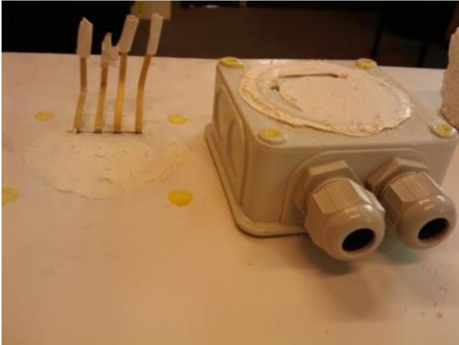
Remove JB of frameless panel (stored in Bay St)
