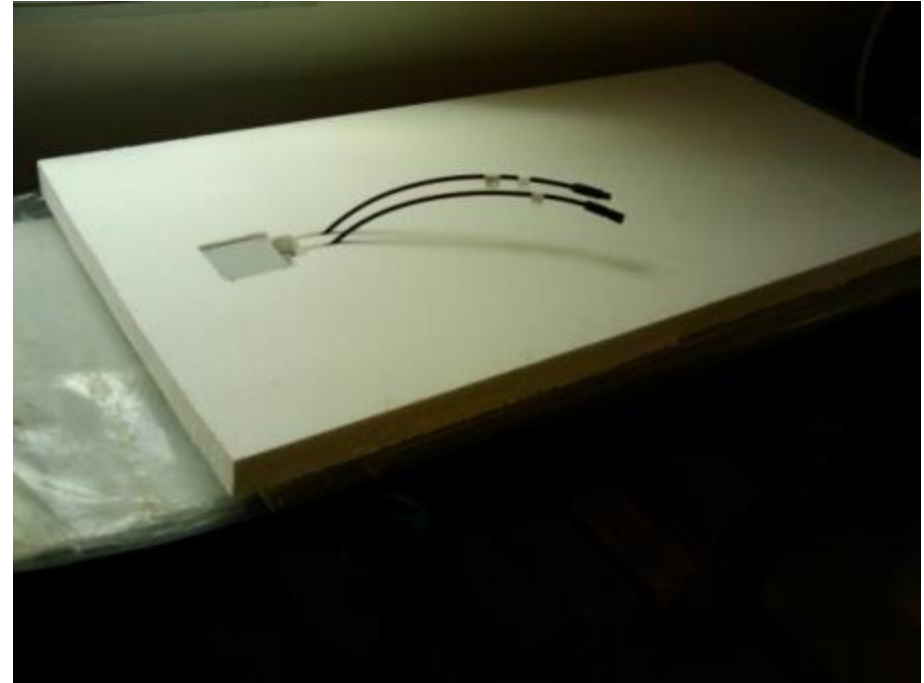
Install back insulation and JB
