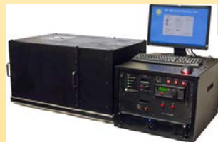
Solar cell simulator for measuring solar cell efficiency
