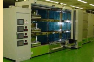
Tube Diffusion & PECVD furnace for p-n junction formation & AR coating
