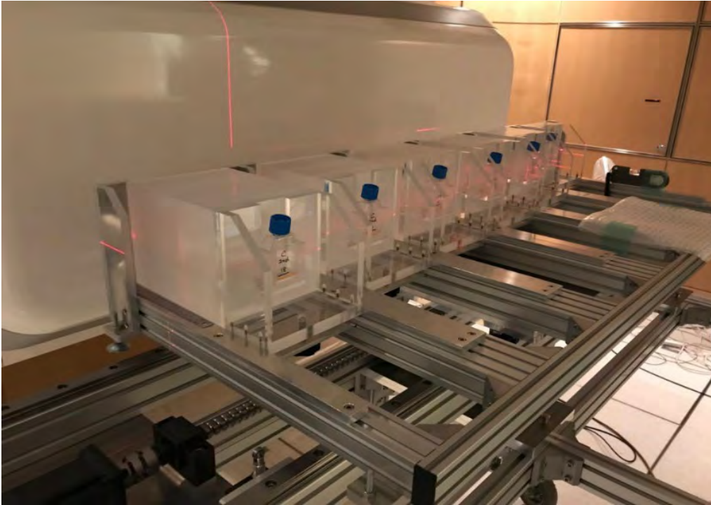
Cell flasks were setup behind PMMA slabs of different thicknesses.
