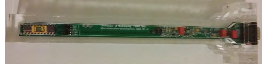
\mu^+ microdosimeter probe in PMMA sheath
