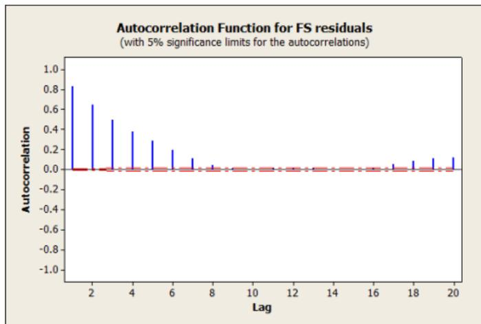
Figure 3: Plotted autocorrelation function (ACF) of the global horizontal irradiation (GHI) deseasoned residuals of Mildura, with 5% significance limits shown in red.
