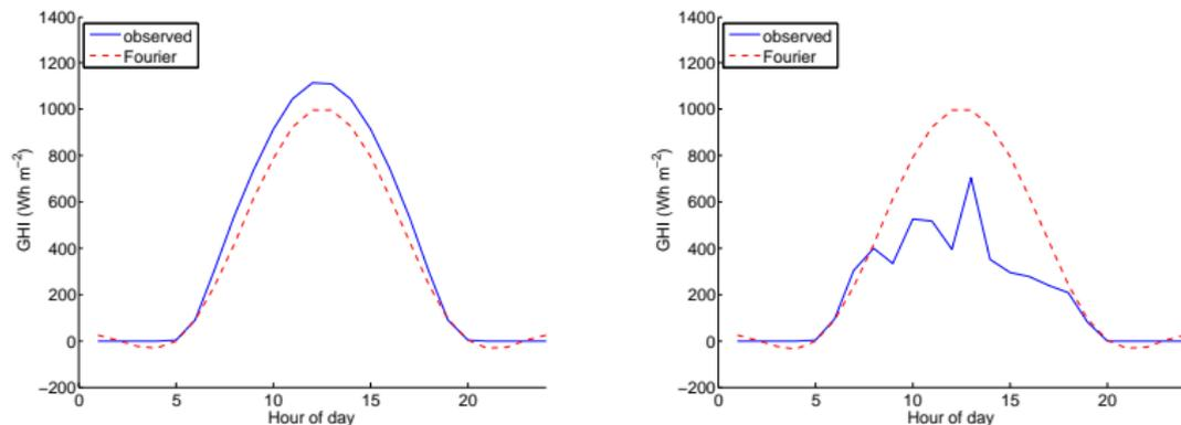
Figure 2: Mildura: observed vs. Fourier global horizontal irradiation (GHI) for a clear sky day on January 2, 2003 (left panel) and a cloudy day on January 1, 2003 (right panel).
