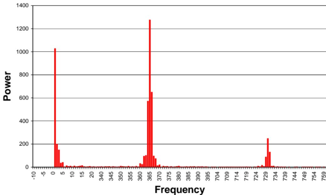
Figure 1: Power spectrum of hourly global horizontal irradiation (GHI) for Mildura. The last three significant frequencies are not shown.
